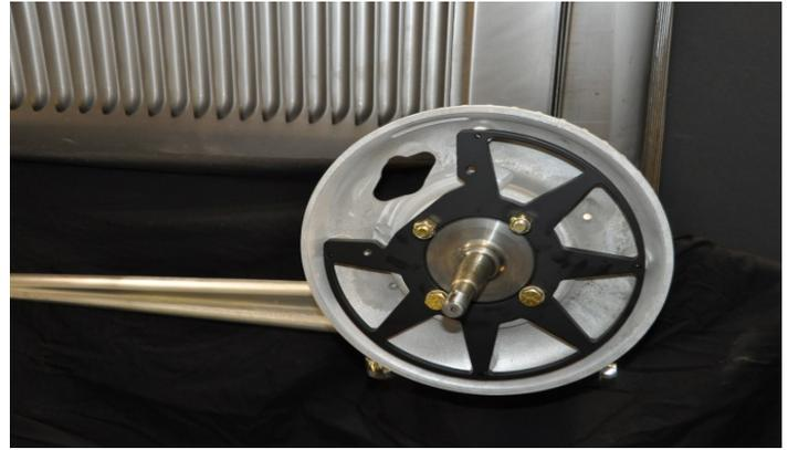
6. Double check that the backing plate slides easily on and off the bracket and has proper clearance to the steering arm.
