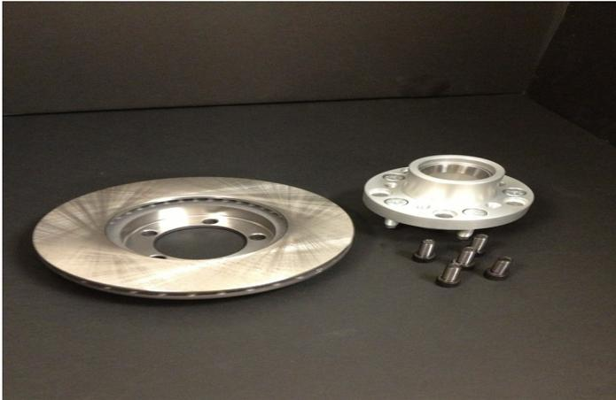
7. Install the rotor onto the back of the hub assembly making sure that the mating surfaces are clean of dust/dirt.
