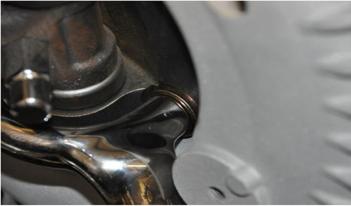
5. Some steering arms may require a spacer between the arm and spindle as shown above to provide proper clearance to the backing plate.
