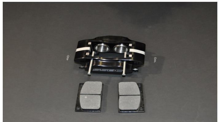
10. Remove the hairpin clips from the two pins in each caliper to install the brake pads. Reinstall clips once the pins are in place with the pads installed.
