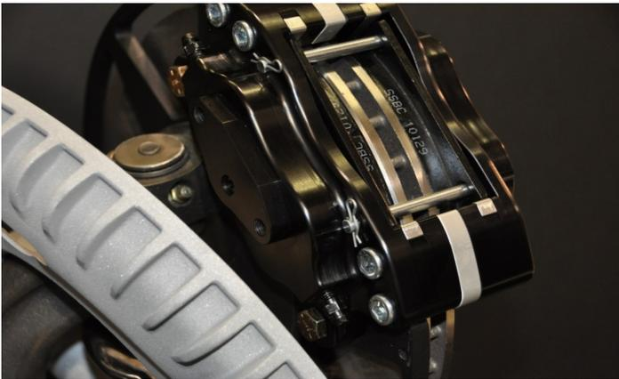
11. Slide the backing plate down the axle to allow enough room to install caliper and bolts. Install calipers using the supplied 3/8-24X1" bolts with lock washers, use a small amount of blue Loctite on each bolt. The left caliper is part #A22225 Right #A22224
