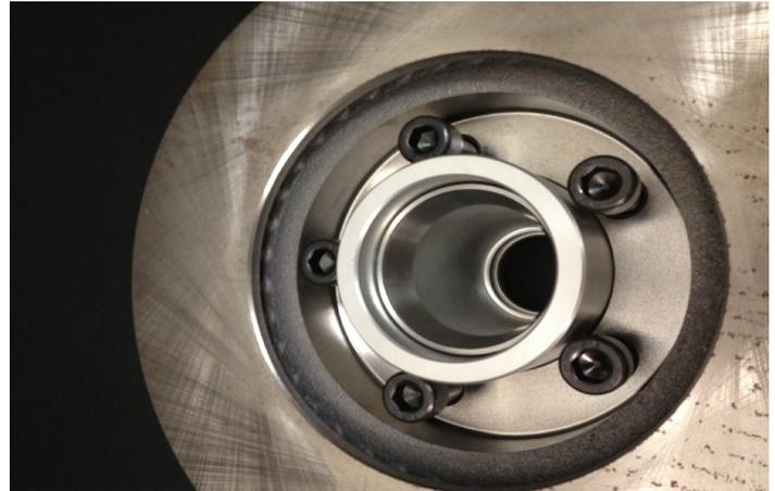
8. Install the supplied 1/2"-20X 1 1/4" socket head bolts, use Loctite on the threads and torque to 85 ft.lbs.
