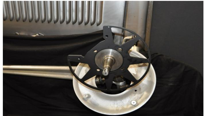
1. Start the installation with the spindles attached to the axle. All brake parts except the rotors are specific for each side and are marked accordingly. If you are working with a final painted or plated axle protect with blue painters tape or by wrapping with a soft cloth. Slide the appropriate backing plate over the spindle and allow to rest on the axle.
