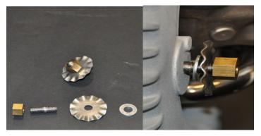
14. Install each stud with the short end into each backing plate, then the spacer, wave washer and brass nut. Use blue Loctite on stud to backing plate and brass nut to stud
