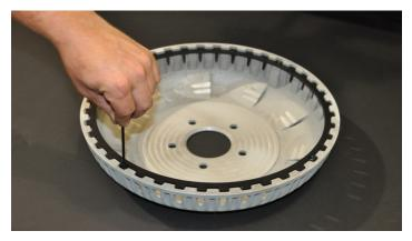
13. Install the painted metal ring into each drum cover using the supplied #10-24X5/8" Countersunk bolts
