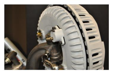
15. Locate the correct dummy wheel cylinder for each side, install the supplied O-ring into each caliper before bolting the wheel cylinder in place with the supplied 5/16X24 Bolts. Use a small amount of blue Loctite on each bolt. The wheel cylinder is 1/8 NPT. Install brake line and any adaptor needed for your application. Install the dummy bleeder valve using blue Loctite (THIS BLEEDER HAS NO FUNCION, DO NOT USE IT TO BLEED THE SYSTEM)
