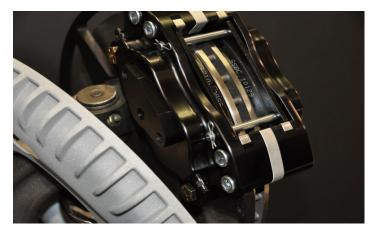
11. Slide the backing plate down the axle to allow enough room to install caliper and bolts. Install calipers using the supplied 3/8-24X1" bolts with lock washers, use a small amount of blue Loctite on each bolt. The left caliper is part #A22225 Right #A22224
