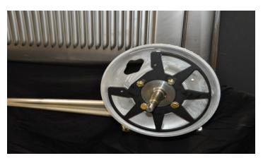
6. Double check that the backing plate slides easily on and off the bracket and has proper clearance to the steering arm.
