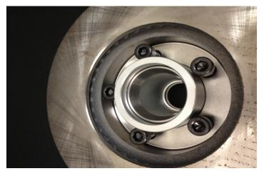
8. Install the supplied 1/2"-20X 1 1/4" socket head bolts, use Loctite on the threads and torque to 85 ft.lbs.
