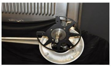
2. Install the caliper/backing plate brackets .Notice each caliper/backing plate bracket is stamped L on one side R on the opposite side. The appropriate mark should be facing out and installed at 12 o'clock. Use 1/2-20 X 1 ½"bolts with washers and nylock nuts on the top two mounting holes.
