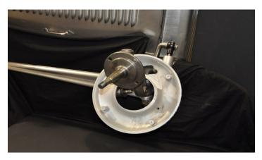
1. Start the installation with the spindles attached to the axle. All brake parts except the rotors are specific for each side and are marked accordingly. If you are working with a final painted or plated axle protect with blue painters tape or by wrapping with a soft cloth. Slide the appropriate backing plate over the spindle and allow to rest on the axle.
