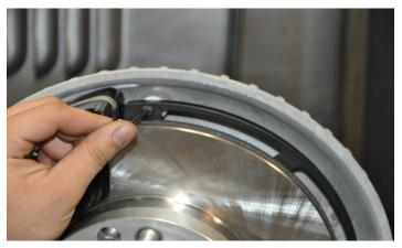
12. Slide the backing plate into position again to double check clearance to caliper, install one #10-24X3/4" Allen bolt to temporary hold into position.
