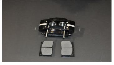
10. Remove the hairpin clips from the two pins in each caliper to install the brake pads. Reinstall clips once the pins are in place with the pads installed.
