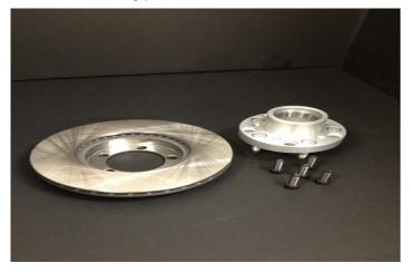
7. Install the rotor onto the back of the hub assembly making sure that the mating surfaces are clean of dust/dirt.
