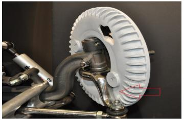
4. Install the steering arms using the supplied 1/2-20X1 1/4" bolts. Some steering arms my require a different length bolt and or a nylock nut as well. At this time slide the backing plate up the axle onto the bracket and check clearance of backing plate to steering arm in the area noted above.
