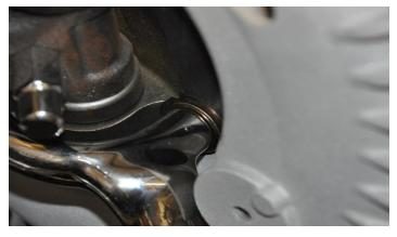
5. Some steering arms may require a spacer between the arm and spindle as shown above to provide proper clearance to the backing plate.
