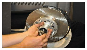
9. Pack the wheel bearings with a high quality grease, install the rear (large) bearing and seal. Slide the rotor onto the spindle and install the front bearing, washer and nut. Preload the bearings and install cotter key.
