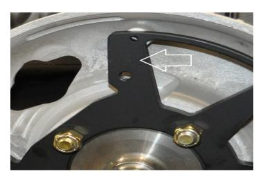
3. Location of stamped mark on caliper/backing plate bracket
